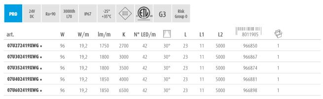
Warning: this strip is 11 mm high. Due to the particular diffusion angle do not use in profiles that are closed with lenses.
